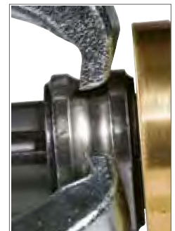
Lock on ball grooves and bearing races.
