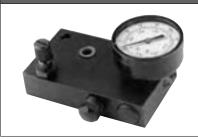
Provides more precise low pressure readings. Remove pressure gauge block and gauge from tester and replace it with this block. Install high pressure gauge from tester (350 bar) onto this new block.
