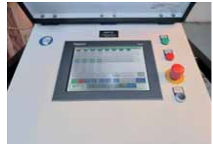
The home screen on the Motion Control System is easy to use and operate. It highlights all activities during use of the Motion Control System. For each cylinder in operation, the cylinders performance is captured and displayed on the HMI screen as illustrated below.
