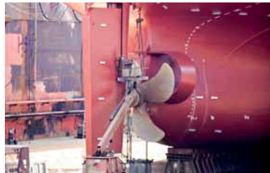
Pictured above: rudder installation for routine maintenance in a dry dock application.
